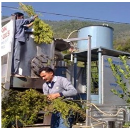
Distillation of essential oil T. minuta
